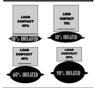
When only partial surface area of bags contact the load—lifting capacity varies in relation to load weight and bag arc.
